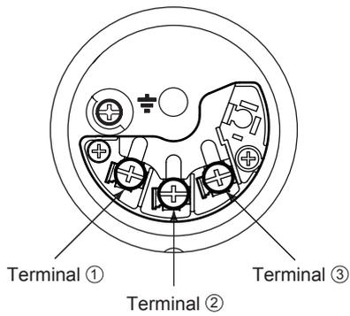
• Terminal Wiring for 4 to 20 mA output, FOUNDATION Fieldbus and PROFIBUS PA communication types
