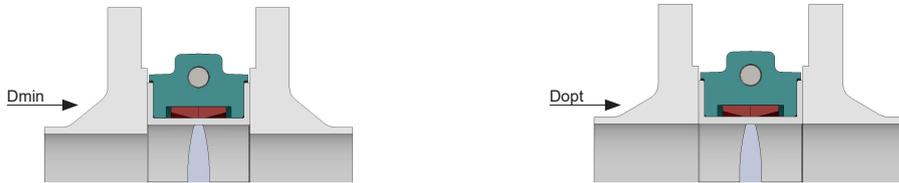
D<sub>min</sub> Minimum diameter of the flange enabling to move the disc (in case of a perfectly centered valve)
